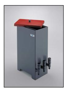
Manual development of films rx up to the format cm 30 X 40 INCLUSED: -2 Fixed compartments 2.5 It for developing and fixing -1 Fixed compartment by 15 It for intermediate and final washing. -W150-V220-Hz50 DIMENSION : Cm 22 x 38 x 53 WEIGHT: 11.5 Kg
